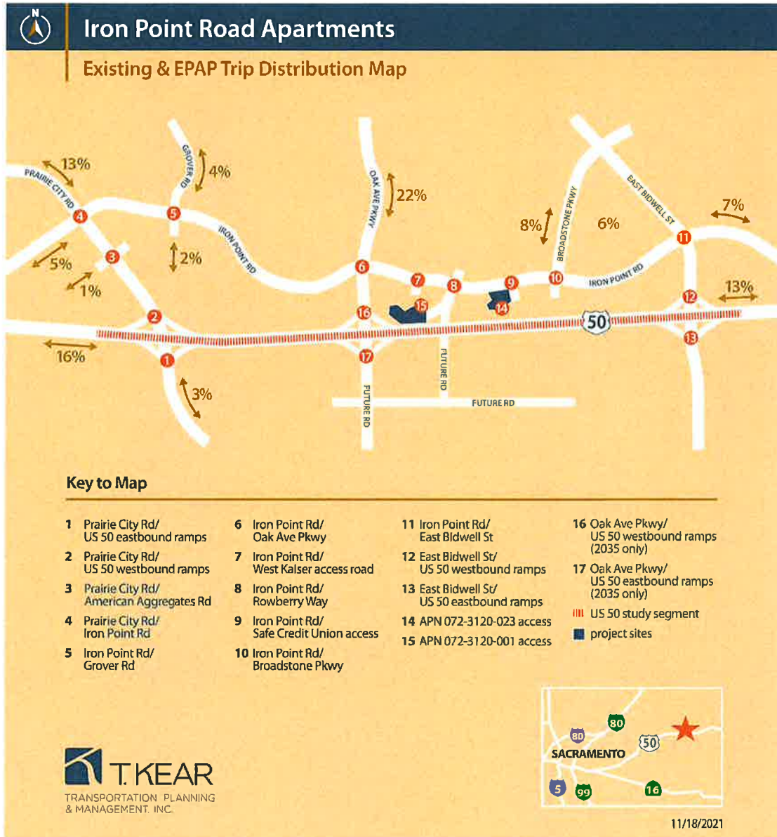
Figure 12. Project Trip Distribution for Existing 2021 and EPAP 2026 Conditions
