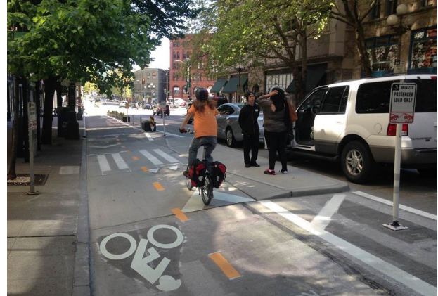
A passenger loading zone allows pedestrians to cross the Class IV bike lane to access the loading island. These designs should also incorporate truncated domes to alert people walking with vision disabilities of the crossing.
