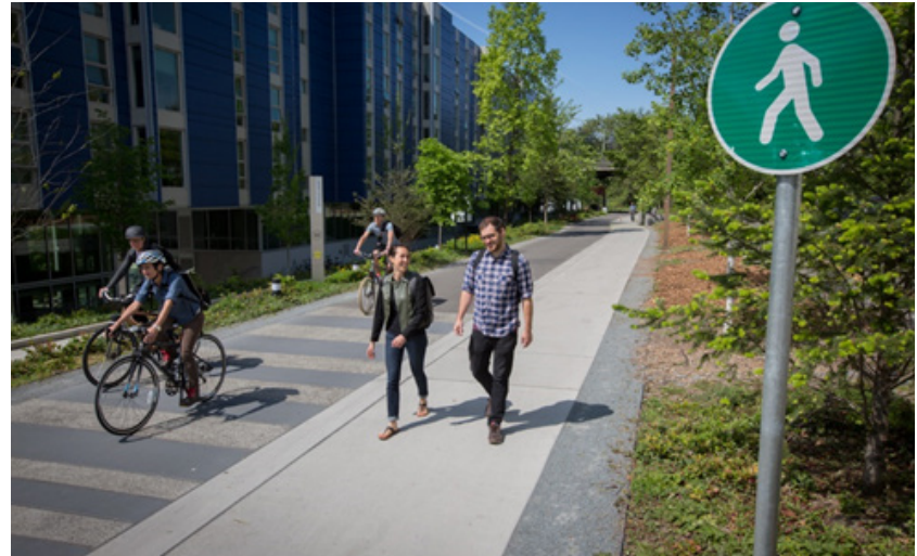
Delineating separate spaces for pedestrians and bicyclists can help alleviate conflict among modes in high use areas. This can be completed through pavement markings or use of different materials to clearly designate space.
