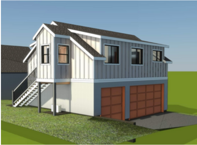
EXTERIOR SIDING COMBINATION BOARD & BATTEN
