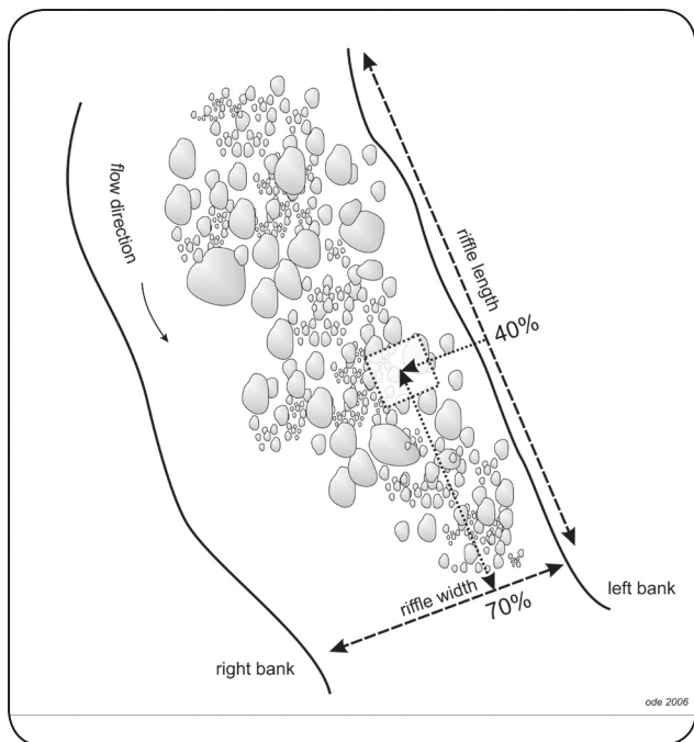
Figure 3. Example showing the method for selecting a subsampling position within a selected riffle under the TRC method. In this example, the random numbers 4 and 7 were selected
