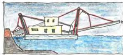
GOLD MINING BARGE, NOTE ANGLED TOWERS AND FORKED CABLE SUPPORTS
