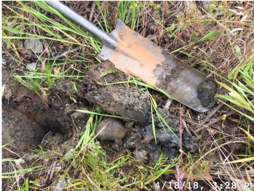
Photo 18: Test pit dug in wetland habitat. High water table observed in test pit.
