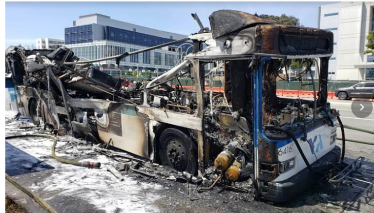
Electric Scooter Caught Fire Onboard the Bus. Bus Hybrid Electric Battery was Intact After the Fire
