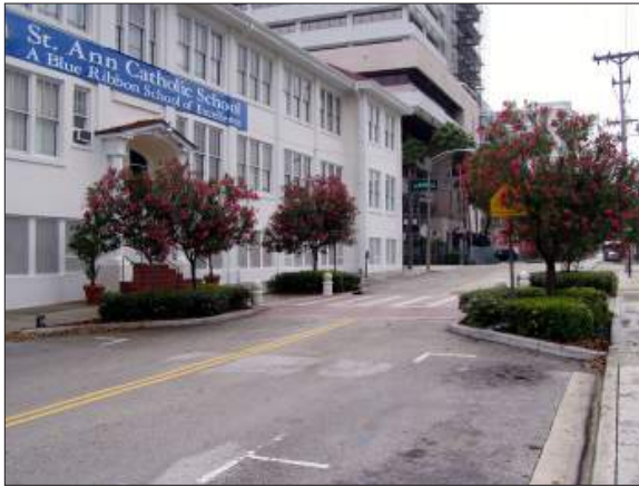
Example of a Mid-Block Bulb-Out
