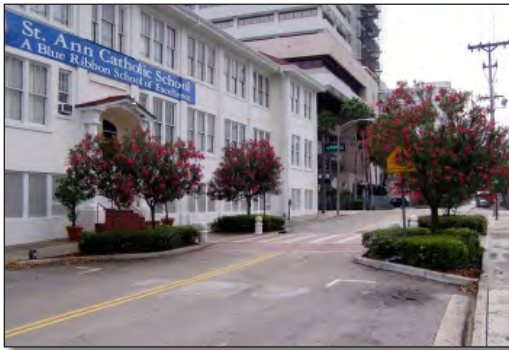
Example of a mid-block bulb-out.
