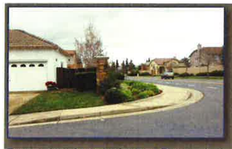
Example of undesirable Corner Lot Street Facing Garage Placement
