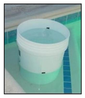
Place a heavy weight in the bucket and add water until the water level inside the bucket is equal with the water in the pool.
