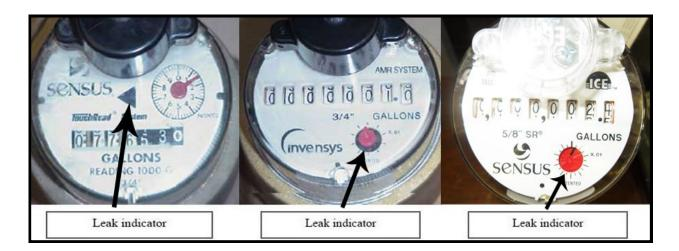
Analog meters have a flow indicator on the face of the meter. These will turn when water is flowing through the meter, even small amounts.
